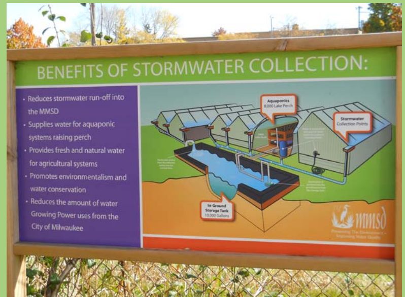
Rainwater is collected and used to raise perch in the stormwater tank. Water is also drawn off for use inside the greenhouse aquaculture systems.
